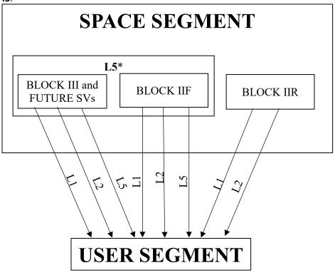
\* Illustration of minimum Signal-in-Space (SIS) components. Future SVs may introduce additional signals beyond those shown.
