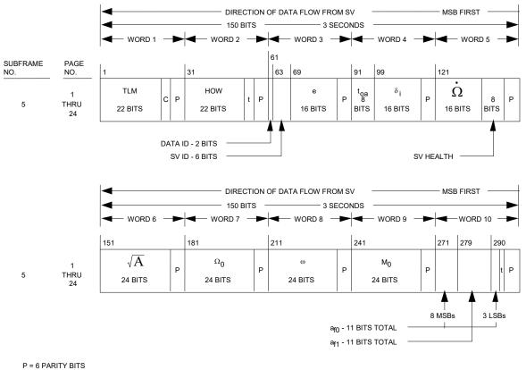
t = 2 NONINFORMATION BEARING BITS USED FOR PARITY COMPUTATION (SEE PARAGRAPH 20.3.5) C = TLM BITS 23 AND 24. BIT 23 IS THE INTEGRITY STATUS FLAG AND BIT 24 IS RESERVED
