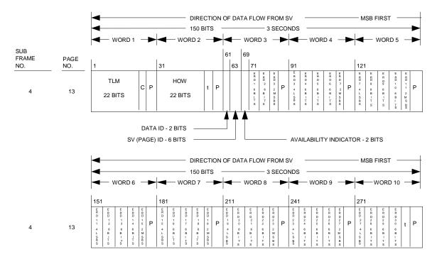
$\mathsf{P}$  = 6 PARITY BITS t = 2 NONINFORMATION BEARING BITS USED FOR PARITY COMPUTATION (SEE PARAGRAPH 20.3.5) C = TLM BITS 23 AND 24. BIT 23 IS THE INTEGRITY STATUS FLAG AND BIT 24 IS RESERVED
