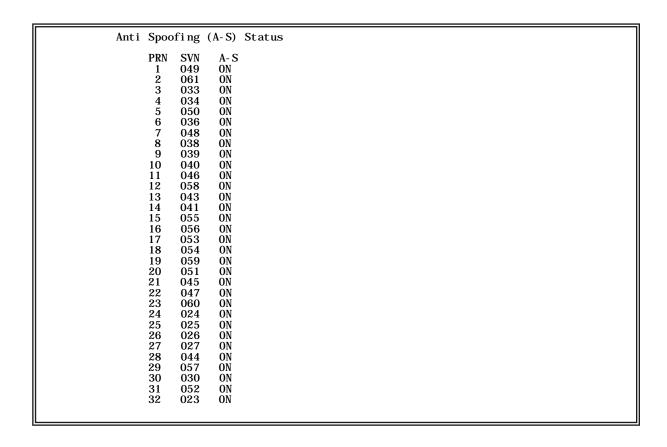
Figure 50-1 Sample of the Anti-Spoofing status file (as.txt)
