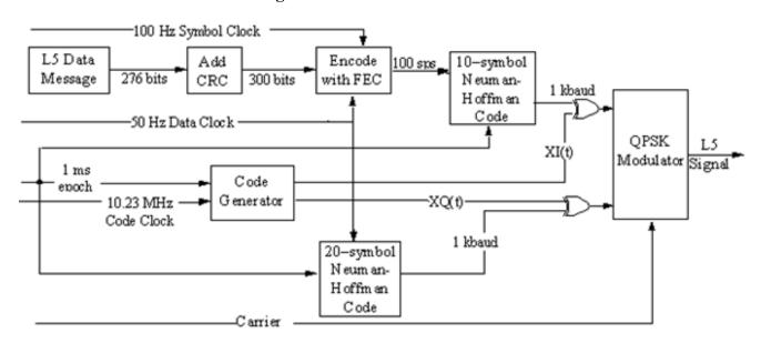
Figure 3-3. Modulation of Signals
