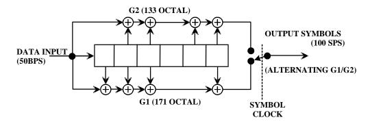
Figure 3-7. Convolution Encoder
