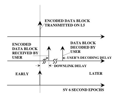
Figure 3-8. Convolution transmit/Decoding Timing Relationships
