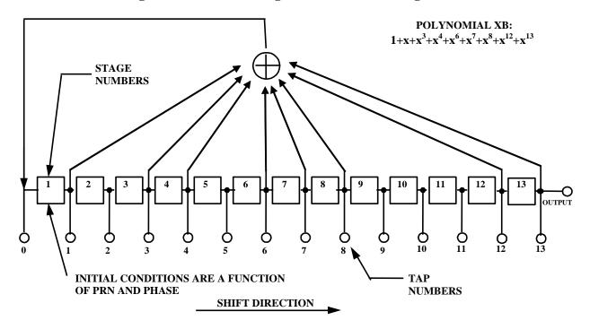
Figure 3-5. XB Shift Register Generator Configuration
