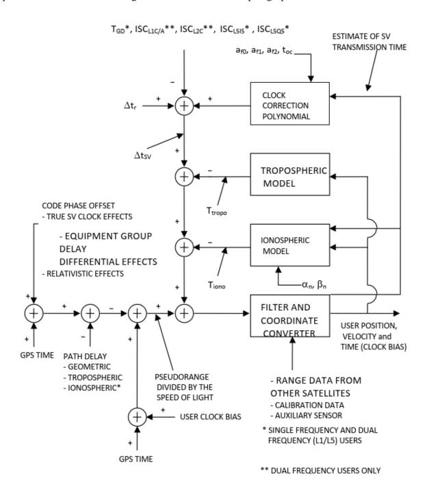
Figure 20-15: Sample Application of Correction Parameters
