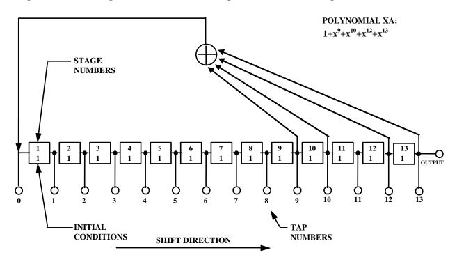
Figure 3-4. XA Shift Register Generator Configuration
