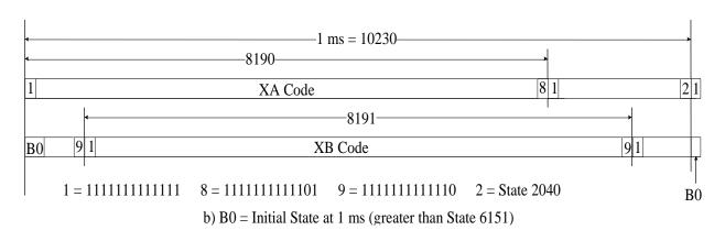
Figure 3-6. Relative Phases between the XA and XB Sequences
