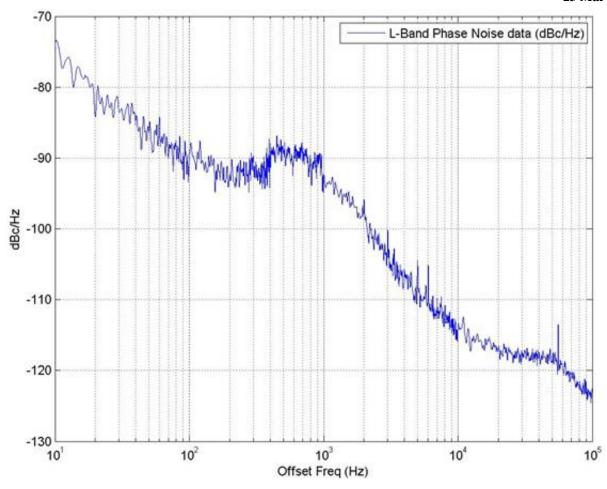
Figure 6-2 Typical GPS III and GPS IIIF L5 Carrier Phase Noise Spectral Density
