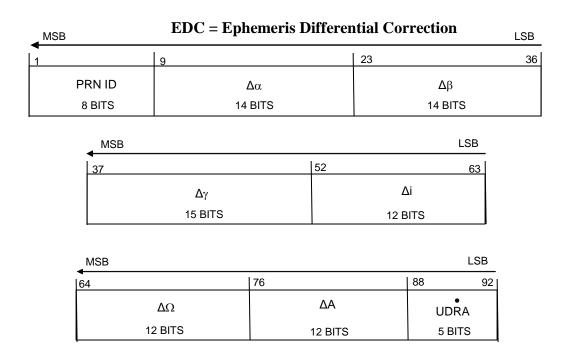
Figure 20-17. Differential Correction Data Packet
