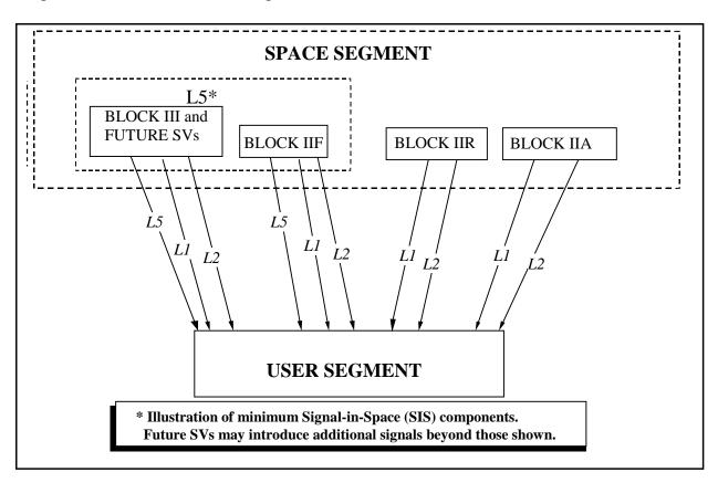
Figure 3-1. GPS Space Segment to User Segment Interfaces
