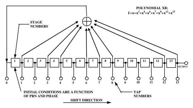
Figure 3-5. XB Shift Register Generator Configuration
