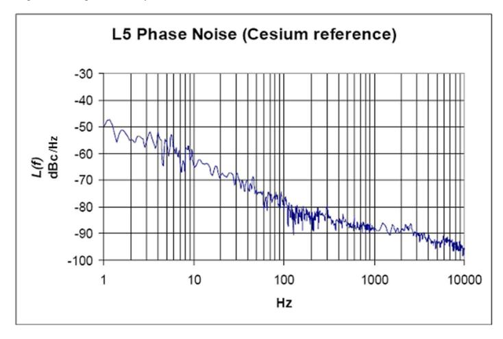
Figure 6-1. Carrier Phase Noise Spectral Density
