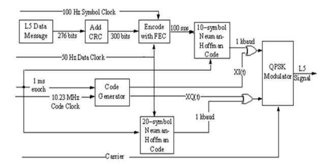
Figure 3-3. Modulation of Signals
