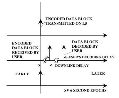
Figure 3-8. Convolution transmit/Decoding Timing Relationships
