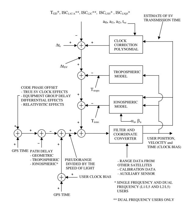
Figure 20-15: Sample Application of Correction Parameters
