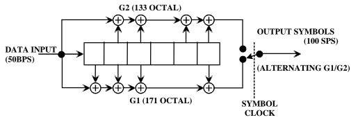
Figure 3-7. Convolution Encoder
