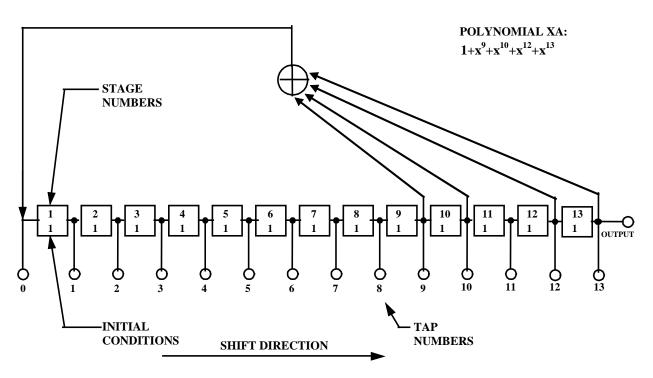
Figure 3-4. XA Shift Register Generator Configuration
