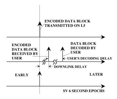
Figure 3-8. Convolution transmit/Decoding Timing Relationships
