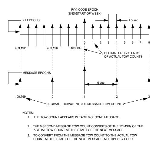
Figure 3-9. Time Line Relationship of a Six-Second Message
