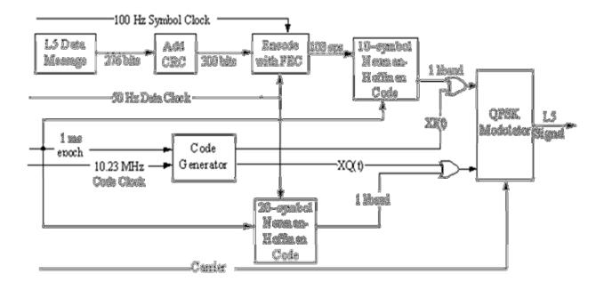
Figure 3-3. Modulation of Signals
