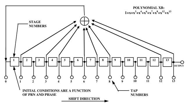
Figure 3-5. XB Shift Register Generator Configuration
