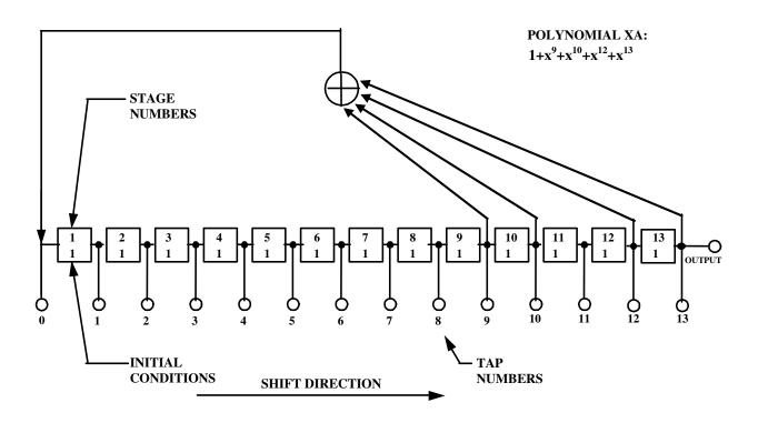
Figure 3-4. XA Shift Register Generator Configuration
