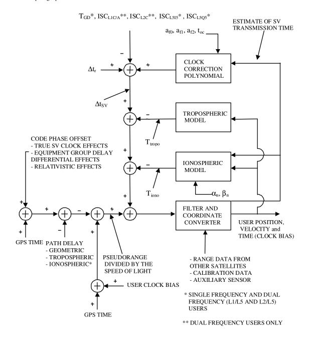
Figure 20-15 Sample Application of Correction Parameters
