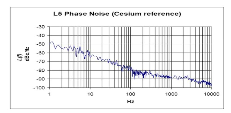
Figure 6-1. Carrier Phase Noise Spectral Density
