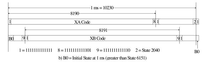
Figure 3-6. Relative Phases between the XA and XB Sequences
