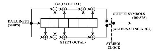
Figure 3-7. Convolution Encoder
