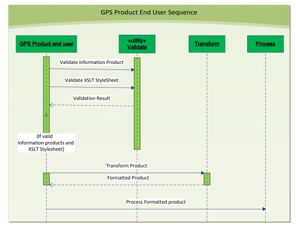
Figure 3-2 GPS Product End User Sequence Diagram
