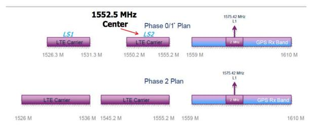
\*Only upper 5-MHz LTE carrier is used in Phase-0. Both 5-MHz carriers are used in Phase-1
