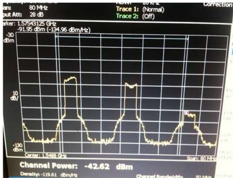
Figure 6-39. Measured Output Power Spectrum of LNA as Measured by JPL at the Holloman Live Sky Test Event
