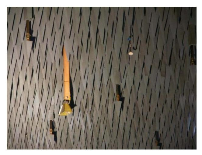
Figure 4. LightSquared Handset Surrogate Antenna (double ridge horn) and the GPS Broadcast Antenna
