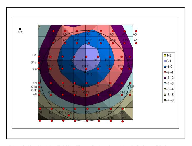
Figure 8. Handset (Double Ridge Horn) Mapping Data, Co-polarization, 1 dB Contours
