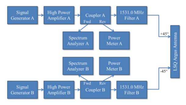
Figure 1 – LightSquared Base Station RF Chains
