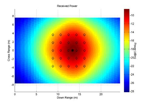
Figure 9 – LightSquared Handset Radiation Profile @ 1632.5 MHz
