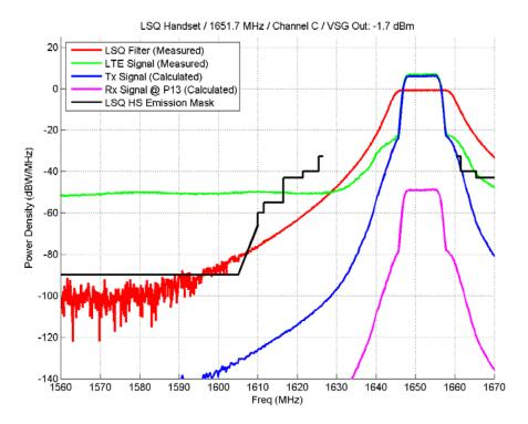
Figure 6 – LightSquared Handset Spectral Validation @ 1651.7 MHz
