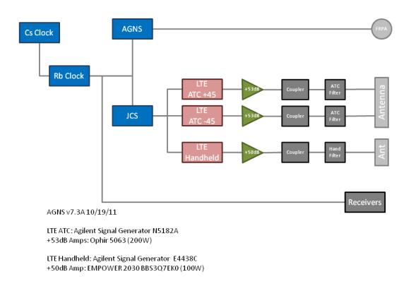
Figure 10 Anechoic Chamber Signal Generation and Timing Set-up
