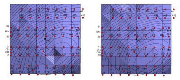
Figure 8 LTE Base Station Mapping, 0.2 dB Contours, +45 (1), -45 (r)
