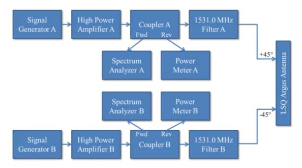
Figure 3 LightSquared Base Station RF Chains
