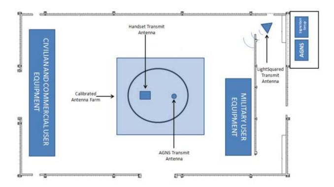
Figure 2 Basic Anechoic Chamber Layout
