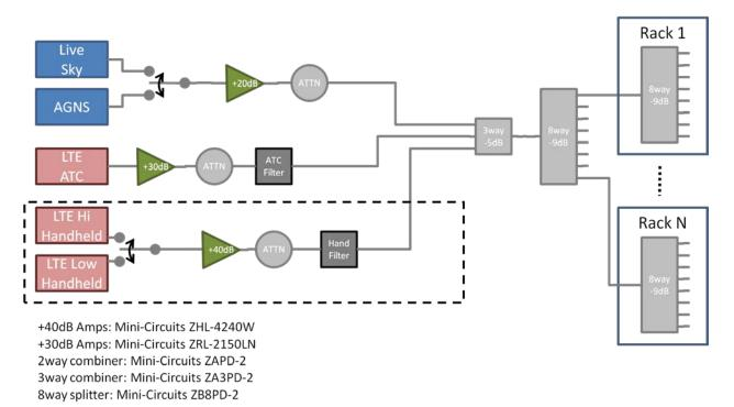
Figure 1 Laboratory Test Set-up
