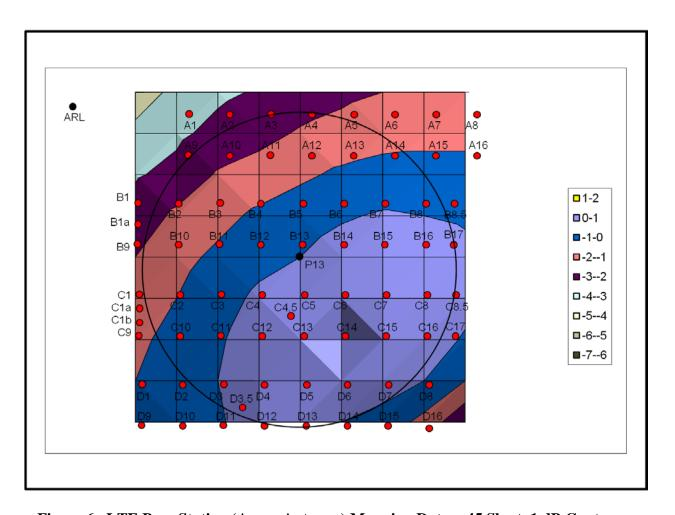
Figure 6. LTE Base Station (Argus Antenna) Mapping Data, +45 Slant, 1 dB Contours
