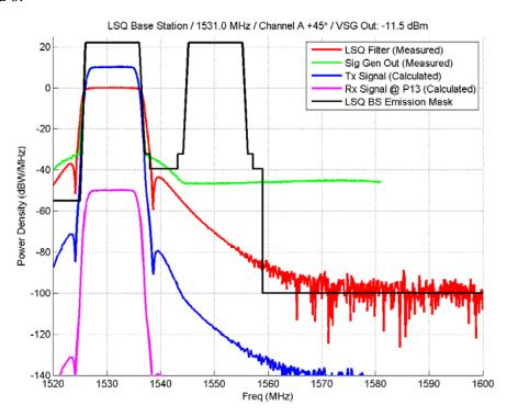
Figure 3 – LightSquared Base Station Spectral Validation +45 Degree Antenna Port
