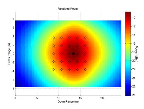
Figure 10 – LightSquared Handset Radiation Profile @ 1651.7 MHz
