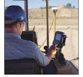
"According to Tom DiGiampaolo, operations manager, an operator on the company's Cat D6M was grading **two building pads per day following stakes**. But after fitting the machine with an automated GPS system, the operator cuts **six pads per day, minimum, with no stakes and no rework**." – Construction Equipment, April 2004
