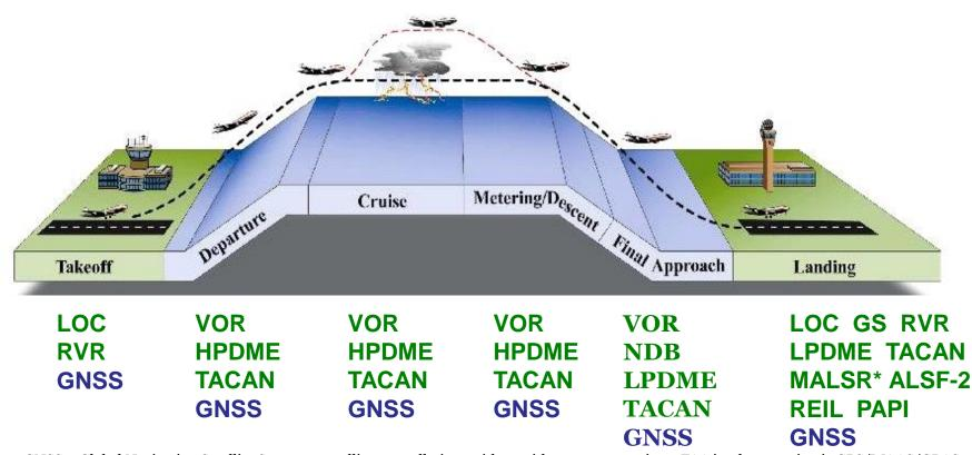
GNSS = Global Navigation Satellite System – satellite constellations with or without augmentations. FAA implementation is GPS/WAAS/GBAS \*MALSR supports CAT I 1/2-mile visibility capability.
