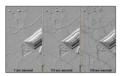
Highly accurate terrain elevation data is replacing older, lower resolution data
