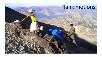
Motions of volcanoes' flanks can indicate the arrival of new magma; GPS is used to monitor changes in activity.
