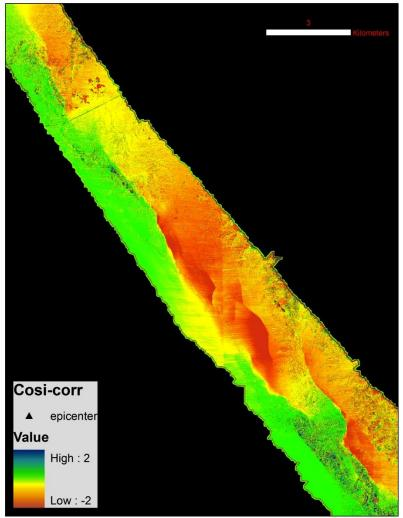
GPS enables ultra-high-precision geo-ref for fault mapping using repeat-pass imagery
