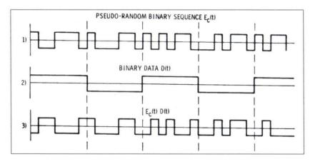
BASE FREQUENCY = 10.23 Mhz L1 CARRIER =  $154 \times 10.23$  Mhz L2 CARRIER =  $120 \times 10.23$  Mhz SATELLITE MINIMUM POWER @ L1 C/A= -160 DBw, L1P=-163 DBw L2 P = -166DBw DATA MESSAGE @ 50 BPS MESSAGE LENGTH = 1500 Bit SYSTEM TIME EPOCHS @ 1.5 Sec Z-COUNT = 403,200/Week DATA MODULO-2 ADDED + CODES
