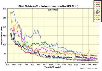
IGS products are formed by combining independent results from each of several Analysis Centers. Improvements in signals and computations have brought the centers' consistency in the Final GPS satellite orbit calculation to ~ 2cm
