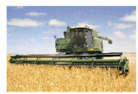
This grain combine can be outfitted with a GPS receiver, yield monitor, and electronic sensors to track crop production based on location. These data can be transferred to a geographic information system to create a yield map and subsequently used to analyze the field and make sitespecific management decisions.
