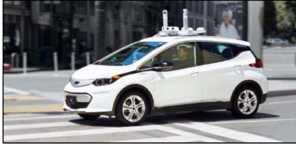
A Chevrolet Bolt is equipped with sensors for development of automated driving (photo courtesy of General Motors Corporation).
