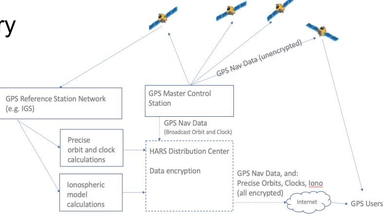
Data encryption and delivery block diagram for a High Accuracy and Resilience Service (HARS). All the components exist except for the HARS-specific encryption and distribution center.
