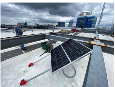
Two geodetic-grade GNSS receiver/antenna pairs at each Test CORS – one pair resilient against Ligado L-band interference, one pair is potentially <u>not resilient</u>. Stations are completely autonomous – solar powered with cellular telemetry.
