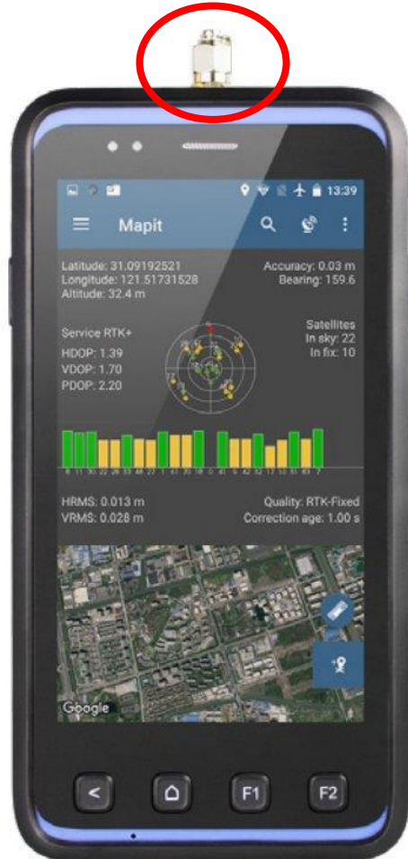
University research uses smartphones for precision GNSS (Source: GPS World Sept, 2018)
