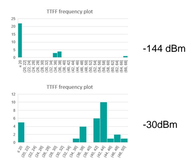
Receiver "X" with 1533MHz interferer (simulating LTE base station) 30 Measurements taken using automated Test Bench
