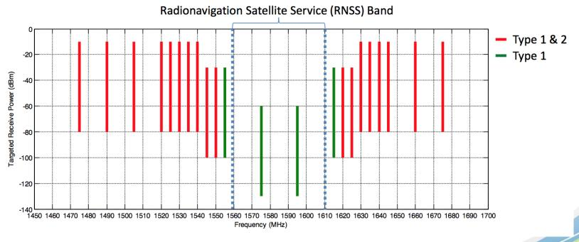
Interference Test Signal Frequencies and Power Profiles
