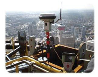
Photo courtesy of WSP Canada Inc GPS HPR receiver used in construction/surveying
