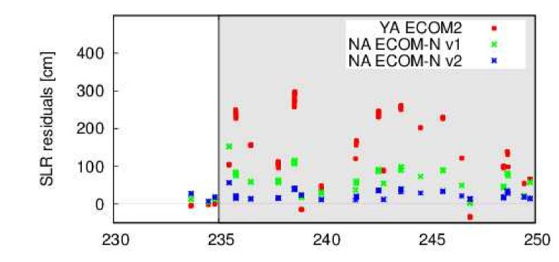
Yaw-Steering SRP (red) is not sufficient for ON mode Experimental ECOM-N... models (green, blue) better represent SRP Additional Challenge: switching epochs between YS and ON are unknown
