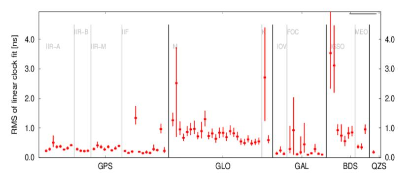
Satellite orbits may also be validated by satellite clock corrections for those satellites which have high-accuracy oscillators. Figure shows the median of the daily RMS of clock estimates w.r.t. linear clock models for different satellite types. Large values indicate modeling problems and/or actual clock quality problems (Prange et al. (2017))
