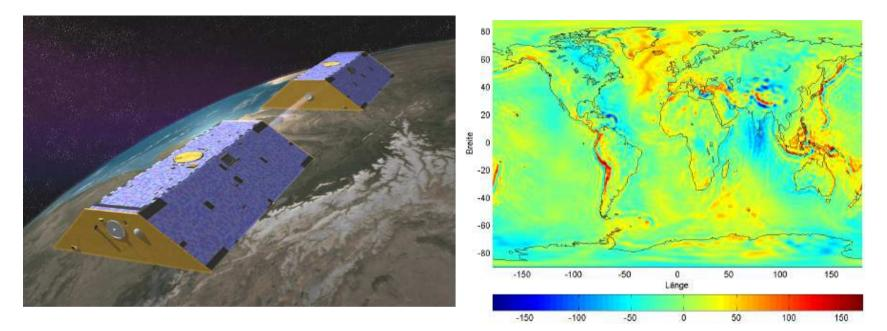
IGS products enable, e.g., precise orbit and gravity field determination – the latter in combination with GRACE inter-satellite link. Left: GRACE twin satellites, right: gravity anomalies from GRACE
