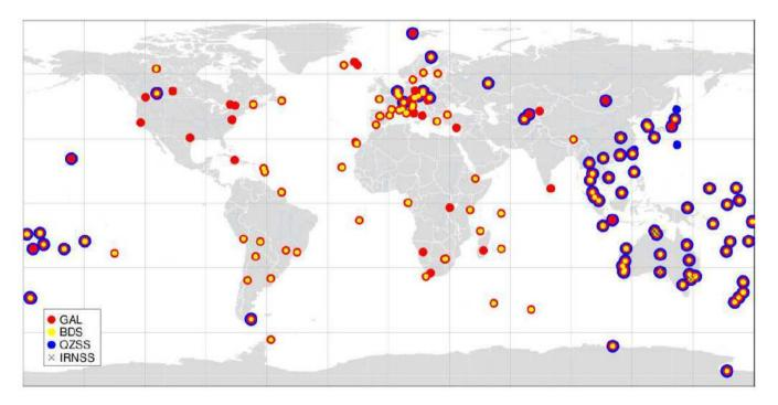
Currently, about 190 Multi-GNSS stations track a combination of Galileo, Beidou, QZSS, in addition to GPS and GLONASS (from Steigenberger & Montenbruck (2017) ).
