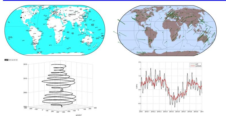
GNSS is fundamental for Earth and atmosphere sciences. From the permanent IGS tracking network (top, left) the ITRF positions/velocities (top, right), polar motion (bottom, left) and variations of Length of Day (bottom, right) are derived. Final IERS products include all space techniques!
