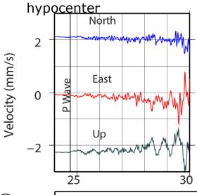
Seismogeodesy detects arrival of seismic *P* (primary) waves used in earthquake early warning to predict arrival and intensity of more damaging *S* (secondary) and surface waves, better than accelerometers alone for large earthquakes, because of magnitude saturation of latter (Crowell et al., GRL, 2013)
