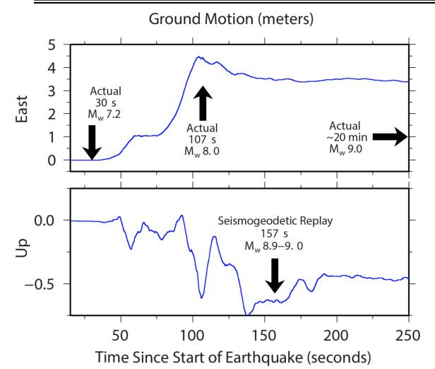
Seismogeodesy improves on traditional seismic monitoring by accurately determining magnitude of large (> M 7)earthquakes without saturation and by estimating both ground motions and permanent displacements
