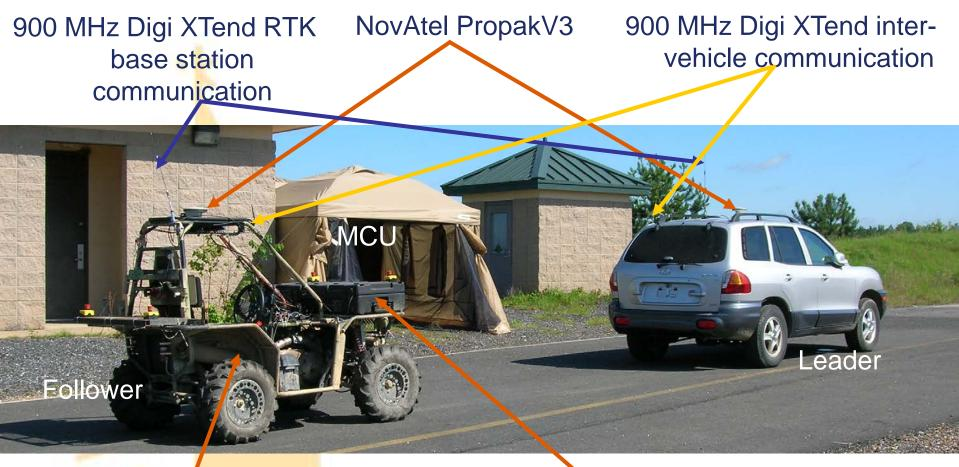
Crossbow IMU440 (under seat) Advantech control and navigation computers Servos Power regulation and distribution
