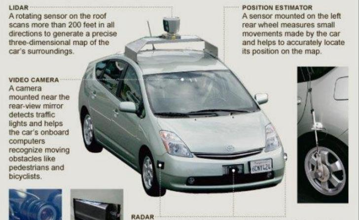
Four standard automotive radar sensors, three in front and one in the rear, help determine the positions of distant objects.
