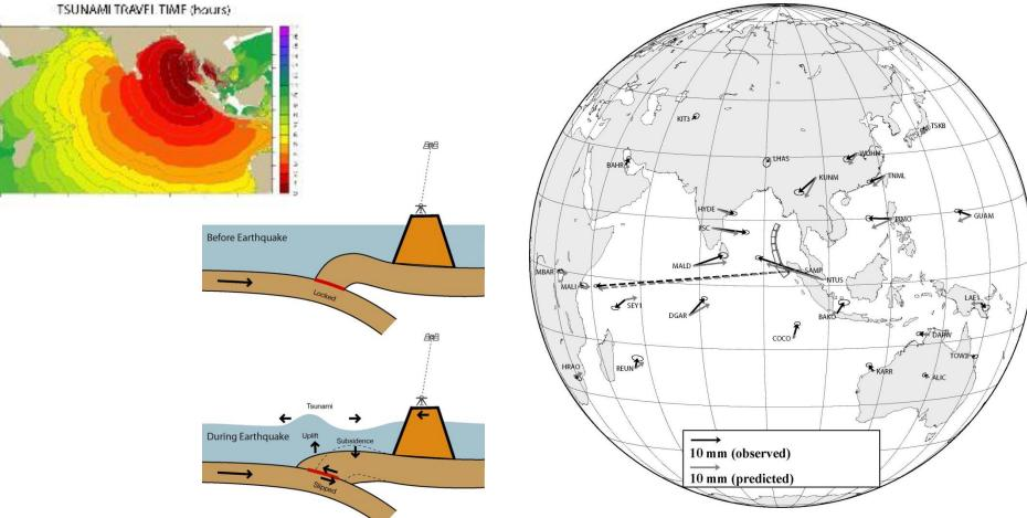
GPS station displacements on 26 December, 2004 observed by the International GNSS Service Network (IGS/GGOS). The largest arrow (SAMP) has been scaled down by a factor of two for clarity. Ref: Blewitt, Hammond, Kreemer, Plag, Stein, Okal, 2009, J. Geodesy.
