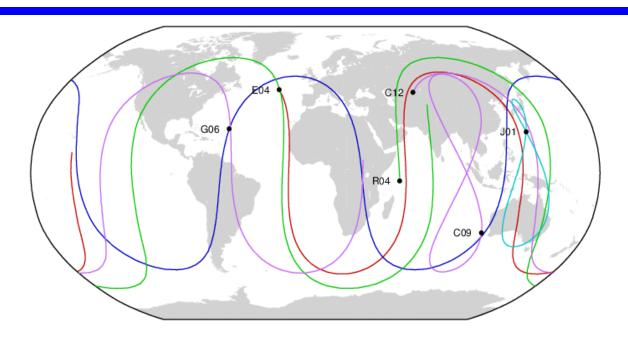
Daily Groundtracks of GPS, GLONASS, Galileo, BeiDou, QZSS (geosynchronous, GPS augmentation).
