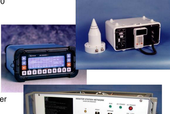
ITT MSN SAASM Receiver 2010 – current L1 C/A, L2C, L1/L2 P(Y) 12 SVs, SAASM
