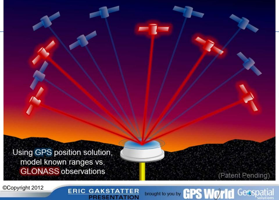
When interrupted, uses modeled GLONASS corrections with GPS to maintain solution
