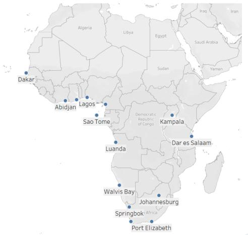
Precise Point Position (PPP) Ground Reference Stations (Coshared between Hexagon AB & OmniStar)
