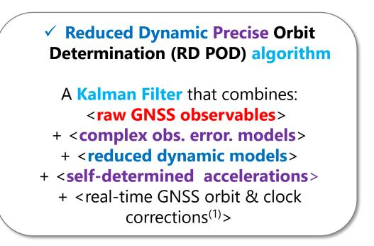
Also allows orbital propagation in the absence of GNSS signals
