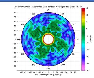
Block IIR-M reconstructed pattern from GPS ACE
