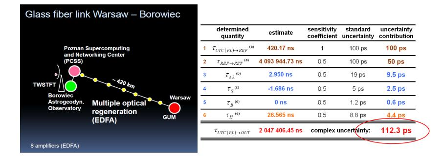
First Operational Optical Fibre Time Link 420 km between UTC Laboratories AOS-PL Combined uncertainty **112 ps**
